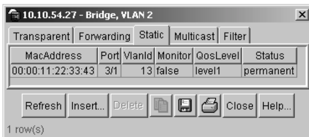
Figure 21 Bridge, VLAN dialog box—Static tab
