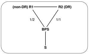
If the BPS is at the edge, then the BPS always forwards traffic on the lowest link of the MLT. Rebooting the DR switch when traffic is flowing through 1/1, forces traffic to recover through 1/2.
